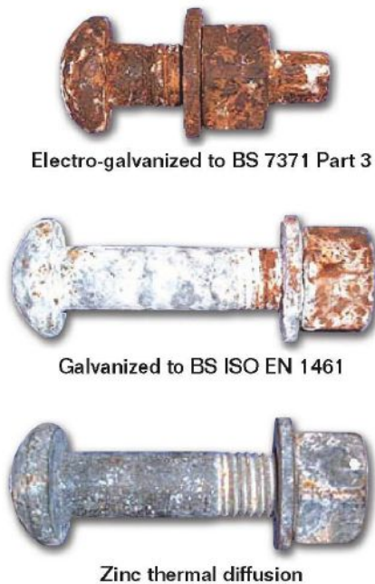
FIGURE 4 Comparison of zinc coatings after 500 h of salt spray testing.
