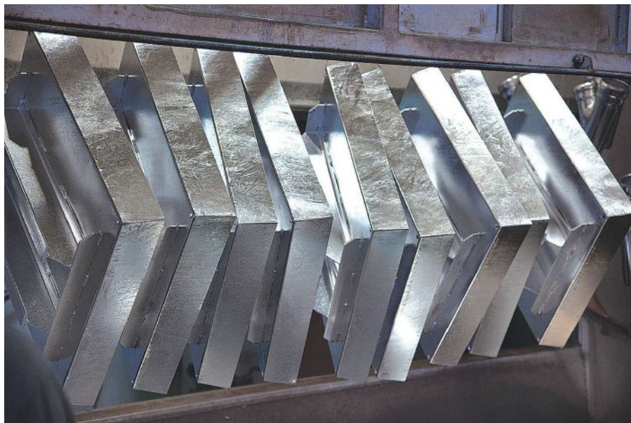
FIGURE 1 HDG of fabricated steel parts.
